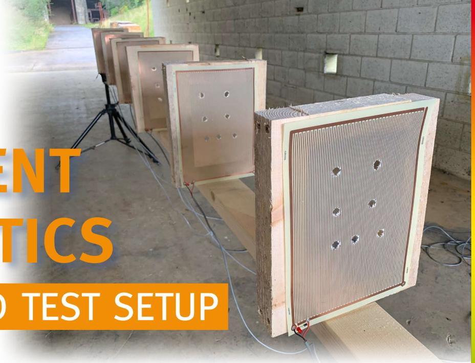
The digital acquisition channels already contain the screen power supply to directly connect the make/break screens. Built-in diagnostics allows to check screens for proper connection to the system and to verify for short circuits at any time. Diagnostic results are displayed via LEDs on the screens and inputs, error warnings in software alert the user.
