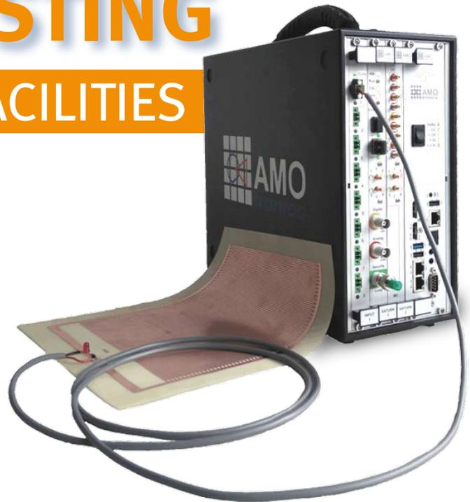
Example: Portable 8-channel fragment test system with make screen power supply and diagnostic features, combined with high-speed analog data acquisition channels in a FlatSaturn unit.
